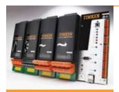
The Commander Unit allows for the control and communication with the monitoring units. The unit includes accommodations for up to 32 channels of shock pulse, 4-20 mA inputs from other sensors, or vibration analysis. The equipment comes standard with four RPM inputs and four digital status outputs but can also monitor units for analog signals and analog output.
